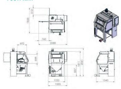
The POSTPRO DP STUDIO is constructed in one compact unit, incorporating the blasting area and cyclone to minimize the machine footprint. It was specially designed to be used for blasting 3D printed polymer parts.
